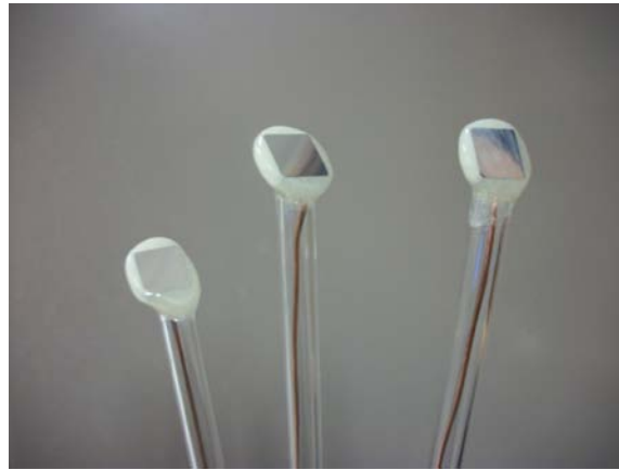
Figure 8: Three electrodes; the metallic area is 1\text{cm}^2
